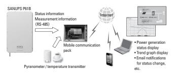
Fig. 7: A connection image of "Mobile Communication Pack"
