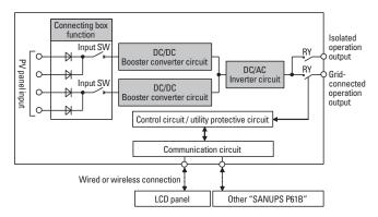
Fig. 4: Circuit block diagram
